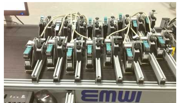
Special Systems: 16 HP Printers on Vacuum Belt
